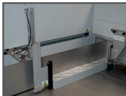
2. Automatic feeding and compression of product piles
