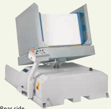
Rear side removal of bad sheets
