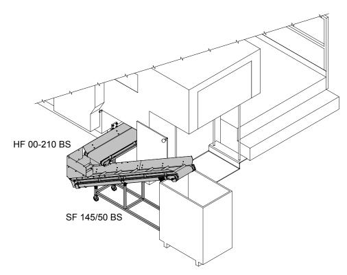
with two conveyors into a container up to a height of 190 cm
