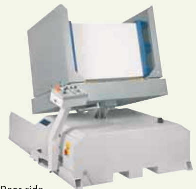
Rear side removal of bad sheets
